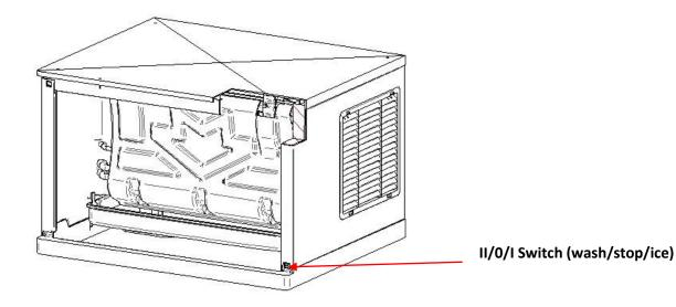
4. Prepare a solution of an appropriate product for the cleaning of ice machines (lime). Do not use hydrochloric acid. We recommend the use of any NSF approved scale removal product. In modular machines the water bucket is filled automatically so we recommend to prepare a previous solution (for example 0.15 gal, according to the manufacturer's instructions with the total quantity of product needed for the water tray 0.8 gal for MS 500 and 1.6 gal for MS 1000 and 0.9 gal for MS 700).
